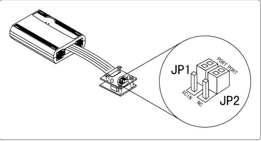
Figure 3.1 Positions of the switches and their factory-settings
